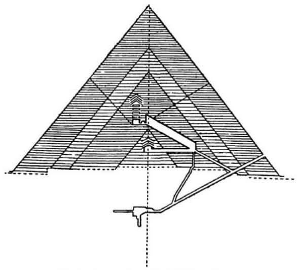
Fig. 7.-Cross-section of the Great Pyramid.
